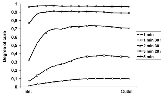
Fig. 6 Evolution of the degree of cure as a function of time along the composite part for two heating zones.
