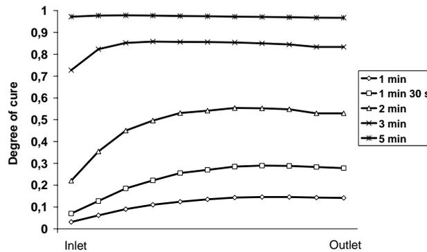
Fig. 7 Evolution of the degree of cure as a function of time along the composite part for three heating zones.
