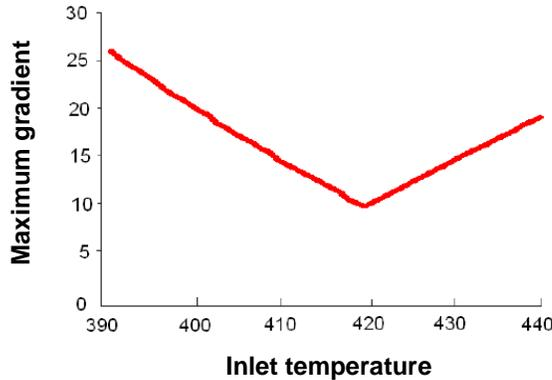
Fig. 4 Maximum cure gradient along the length of the composite part as a function of the inlet temperature for two heating zones (recall that a mean mold temperature of  $390^\circ\text{K}$  was selected).
