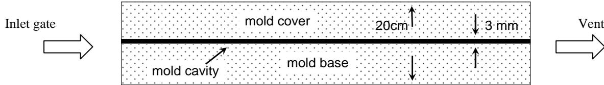
Fig. 1 Vertical cross-section of a typical rectangular mold.
