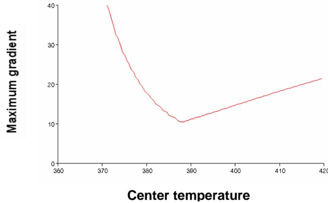
Fig. 5 Maximum cure gradient along the composite part as a function of temperature in the center of the mold for three heating zones.
